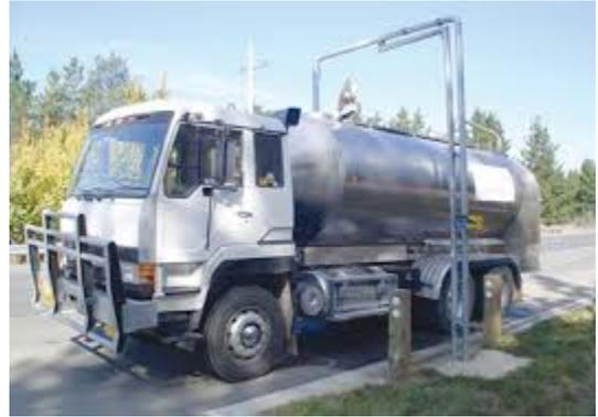
A standpipe is a freestanding pipe used to provide running water in areas with no other water supply. In the case of EPCOR, the pipe will deliver measured amounts of water for fill of mobile water tanks used by water haulers or private parties. The photo with the water truck depicts a typical standpipe facility. The EPCOR facility will have two outlets and be able to fill two trucks at the same time.
